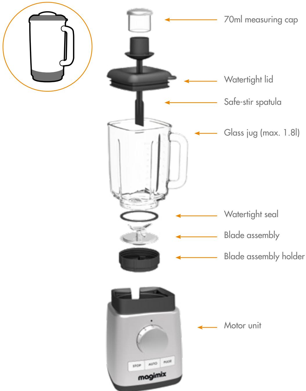
Carefully wash all the parts (except the motor unit) before using for the first time.
